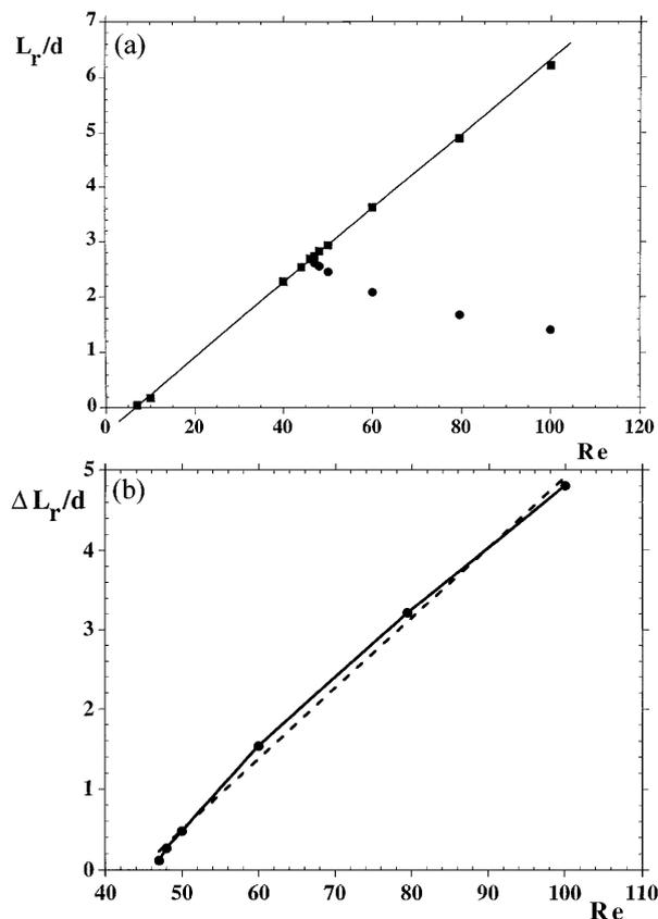
FIG. 2. Reynolds number dependence of (a) the length of the recirculation zone  $L_r/d$  (unconfined circular cylinder). Circles: mean value; squares: basic flow. (b) The decrease of the recirculation length  $\Delta L_r/d$ . Solid line: best power law fit; dashed line: best linear fit.
